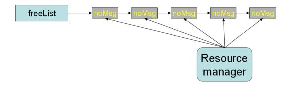
When a thread needs to send a message, the resource manager takes the next free message object in the freeList of the corresponding RTController object and returns it to the controller that will fill in all message information and send the message. If there is no free message in the list, a new bunch of messages are allocated in the system heap with the call to the function
