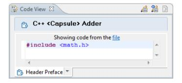
The header preface code snippet will be copied verbatim at the top of the header file that is generated for the capsule. If you only need to use the included file in the capsule implementation file, you can instead add the #include in the "Implementation Preface" code snippet.
