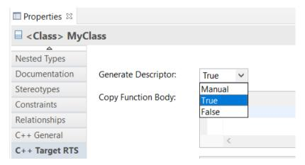
If you set the property to "False" no type descriptor will be generated for the type. This means that you for example cannot send an object of this type by value with an event (since the RT Services Library does not know how it shall be copied). Another thing that is lost is the ability to print an object of this type to the log using the Log service (since the RT Services Library does not know how it shall be encoded).
