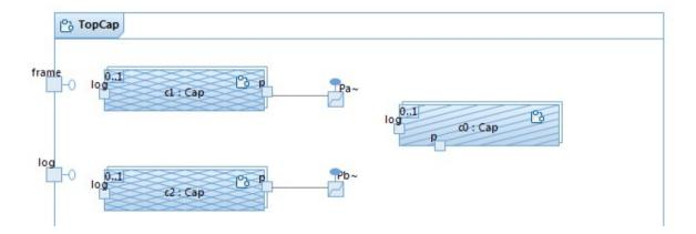
The capsule "TopCap" has an optional capsule part "c0" and two plugin capsule parts "c1" and "c2". All capsule parts are typed by a capsule "Cap". The "TopCap" capsule may contain the following code:
