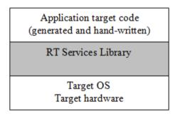
The RT Services Library isolates the application code from the target environment, so that the same real-time application can be built for multiple target environments. In addition to providing this platform independence, the RT Services Library also provides certain services which the application can use at run-time. The following categories of services are provided:
