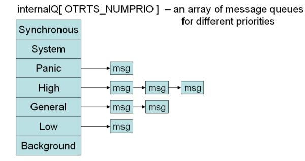
As can be seen in the picture the queue is categorized according to priority level to ensure that messages with higher priority get dispatched before messages with lower priority.
