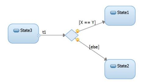
When the trigger t1 has fired and executed its effect, then the guards of the transitions that leave the choice point are evaluated. If X equals Y then the transition is taken to State1, other-
