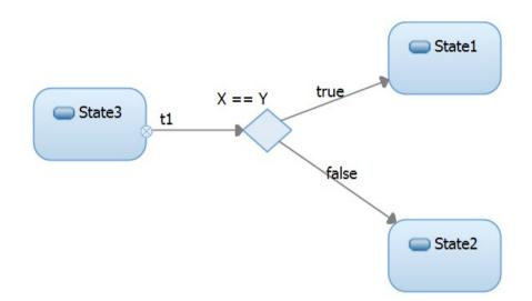
When trigger t1 fires, if X equals Y then the state machine transitions to State1, otherwise to State2. A limitation with this approach is that there can only be two exit paths from each choice point.
