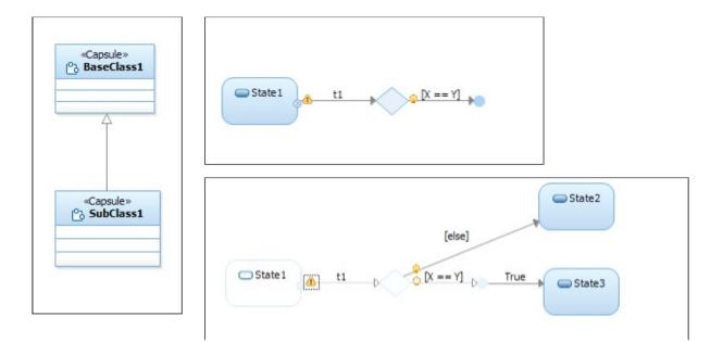
So, the pattern for importing choice points from RoseRT to Model RealTime is as shown below. A transition to a junction point is added to hold the choice point condition.
