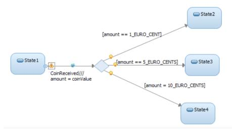
This state chart describes a vending machine. When the CoinReceived trigger is fired we want to go to some state based on the value of the coin that was entered. The order in which things happen is:
